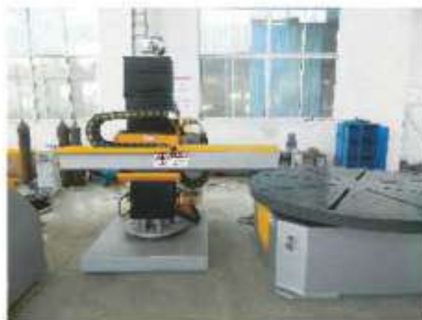
焊接操作架 Welding manipulator
