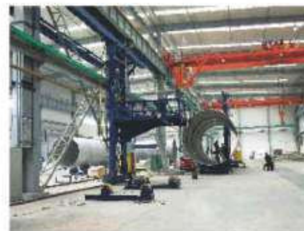
悬臂焊 Cantilever welding
