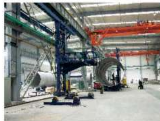
悬臂焊 Cantilever welding
